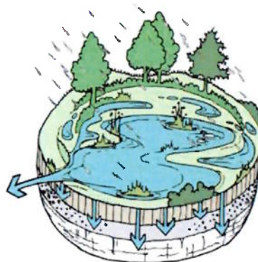
Surface flow rates are small at first, but increase with higher intensity rainfall events. The volume of runoff will generally be greater with increased rainfall intensity and duration.
